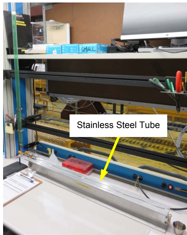
Figure 9-2: Set-up for Water Penetration Test (Actual Sample)
