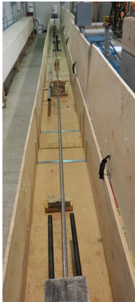
Figure 6-2: Set-up for Creep Test (Actual Sample)
