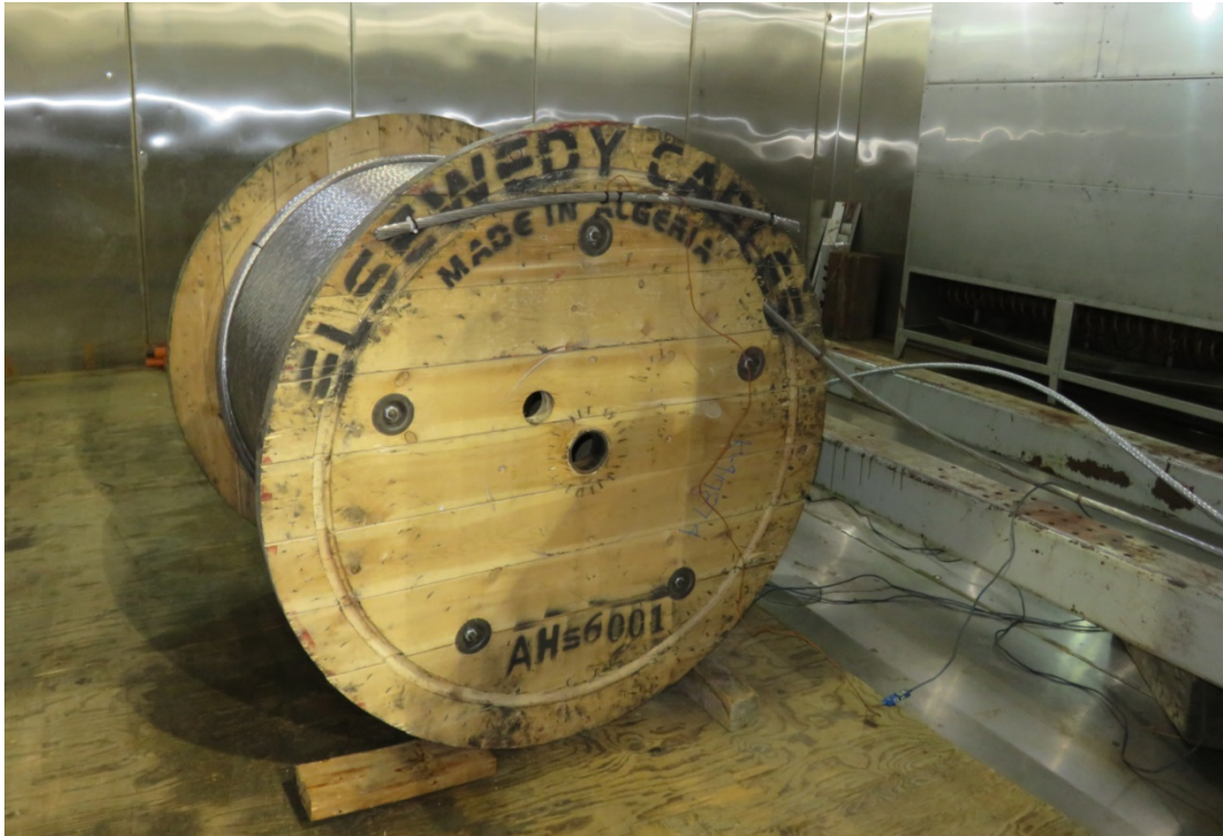
Figure 8-1: Set-up for Temperature Cycle Test
