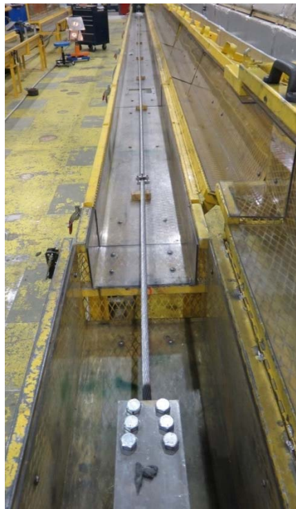
Figure 3-2: Set-up for Stress-Strain Test (Actual Sample)
