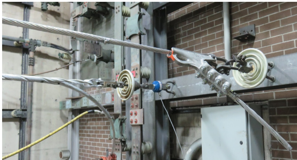
Figure 10-3: Set-up for Short Circuit Test (Actual Sample)
