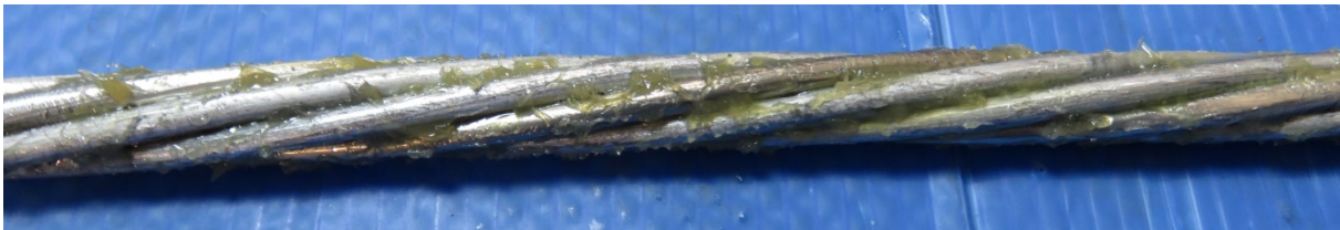
Figure 10-9: Short Circuit Test Dissection: West Section – 2 nd (Inner) Layer with Grease
