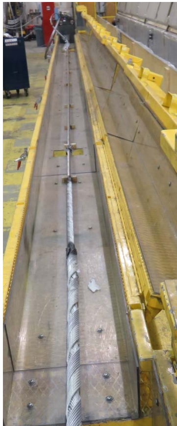
Figure 2-2: Set-up for Tensile Performance Test (Actual Sample)
